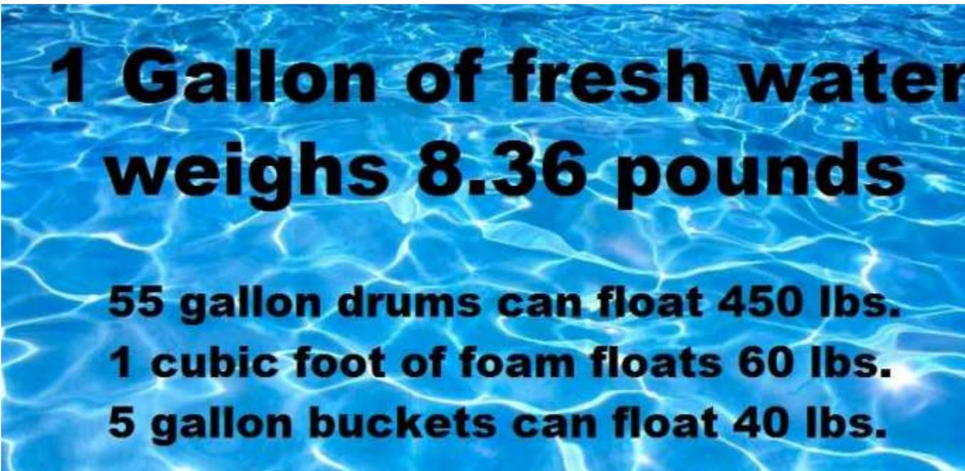
For each gallon of water displaced by flotation materials you will gain about 8 lbs of buoyancy. This is the force that causes objects to float. By dividing 1800 lbs by 8lbs we calculate that 225 gallons of water needs to be displaced. You can use 4 55 gallon drums, eight 30 gallon drums, 30 cubic feet of foam, 45 5 gallon buckets or 225 one gallon milk jugs.
